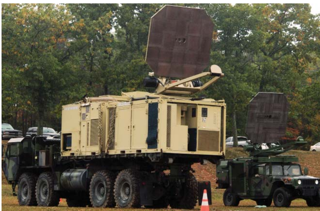
Copyright US Marines/Joy E. Crabaugh. Two US Marine Corps vehicles mounted with the Directed Energy Active Denial System, a non-lethal weapon that uses directed energy. When fired at a human, it delivers a heat sensation to the skin and generally makes them stop what they are doing and run.
